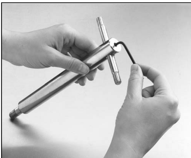
Figure 9. Tightening setscrew with hex key.
